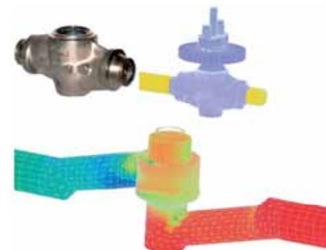
Code_Saturne/Code_Aster chaining on an Alstom-Velan glove valve : mesh and internal fluid pressure field.
