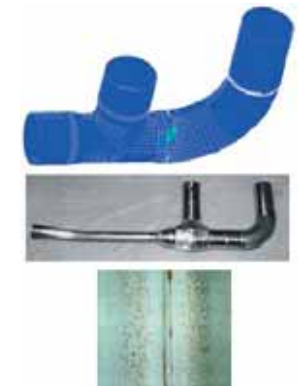
RRA circuit elbow : damage calculation by the Dang Van criterion and thermal crazing.
